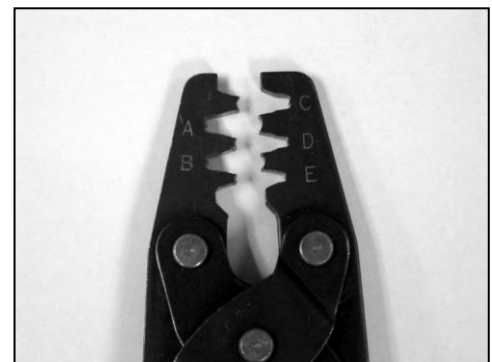
Figure 3.1 Rolling crimper. (Radio Shack P/N 64-2983 or equivalent.)
