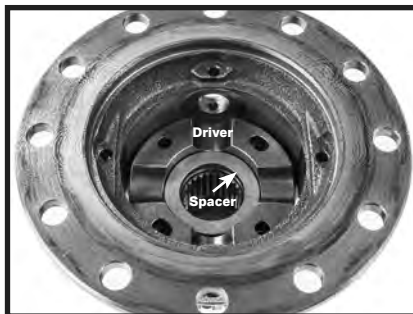
Figure 6: Driver goes onto the side gear, teeth meshed, then spacer is set in middle.
