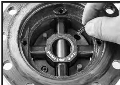
Figure 7: Set pinion shaft block in center, install pinion shafts. Then install small parts into driver using some grease to help hold them in place.
