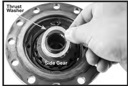
Figure 9: Set second side gear onto driver, making sure to mesh teeth with driver. Set second thrust washer shiny side down so it rests against side gear.
