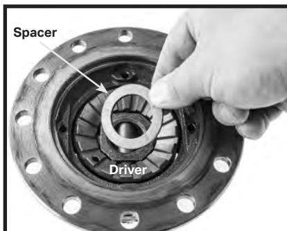
Figure 8: With second driver now installed, set second spacer into center.
