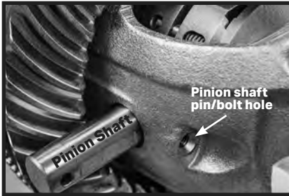
Figure 9: Install pinion shaft, then pin/bolt
