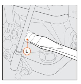
B) Now adjust the idle mixture (idle quality) using the idle needle screws (see J) with the engine at normal operating temperature, the air cleaner in place, the throttle fully closed and the choke fully open (see K). Turn the idle screws IN (clockwise) to provide a leaner mixture and OUT (counterclockwise) to provide a richer mixture.
